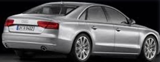
2011 Audi A8 ASF all aluminum except the B-pillars Source: Audi
